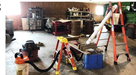
Test2 – vacuum collection system simulation.
