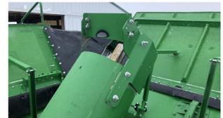
John Deere S790 Grain Tank clean grain auger bearing
