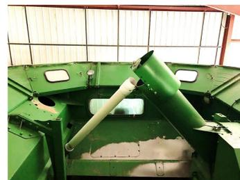
PVC pipe placement in grain tank.
